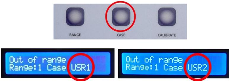
The value of the reference element is saved in the non-volatile memory of the device (EEPROM), so you can use this value the next time you use the meter.
