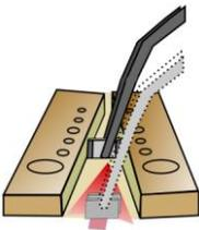
The calibration jumper should be placed in the measuring socket by the tweezers as shown in the picture. The element's contacts should adhere to the connector's contact bars (wedging between the bars), and the element itself should **be placed vertically**. Move the tweezers away from the connector before performing the calibration.
