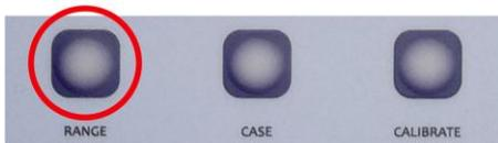
**WARNING:** When measuring very small values, it is recommended to turn on Range 1. Do not use Auto mode, because the accuracy of the measurement decreases in this mode.
