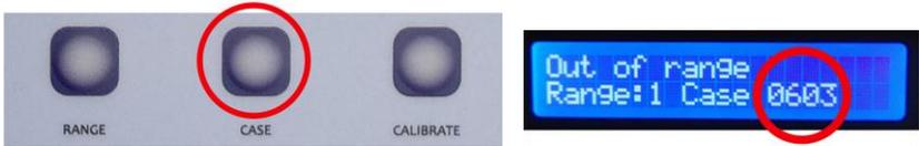
3. Insert the calibration element of the above size (0603). This element (jumper type) is provided with the equipment.
